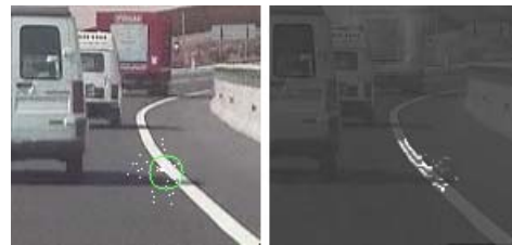
Figure 2: Swarm perception. A swarm created in a white region will be attracted by white colours on high gradient magnitude pixels, shown brighter on the image on the right.
