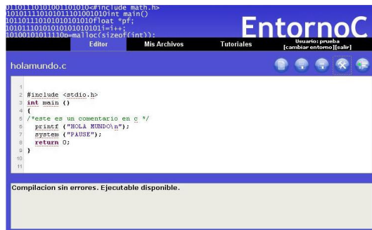
Fig. 2. OLC Work screen. With the tabs menu, the tools bar, and two text areas: one for the code and the other one for the results.
